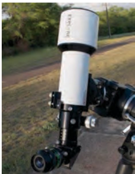
Image 4 - Graduations on the focuser shaft allow quick return to focusing when changing eyepieces. The right-hand focusing knob has two speeds for adjusting the focus.
