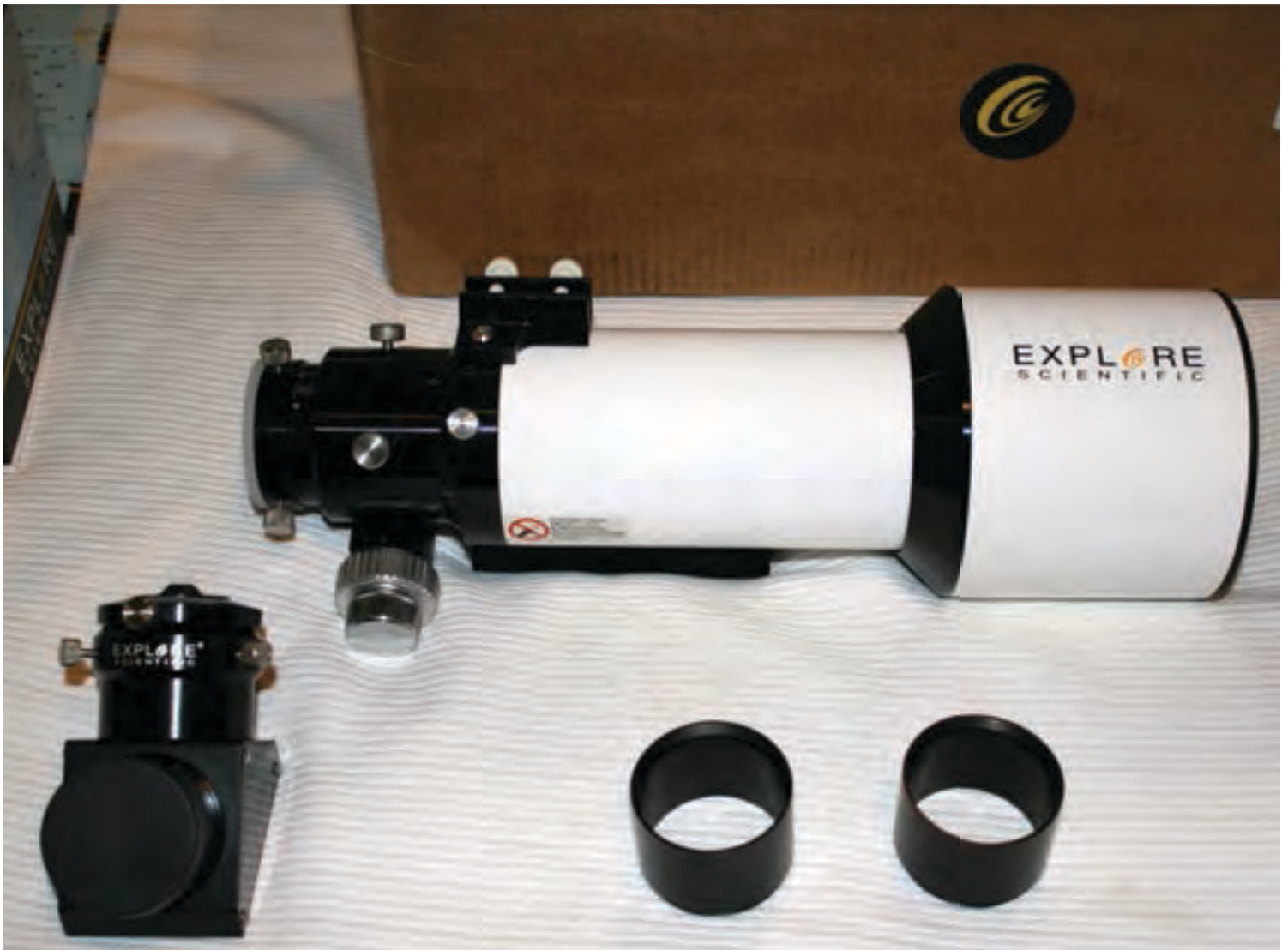
Image 3 - The ES80 comes with a 2-inch diagonal, two focuser extension tubes for astrophotography, a 2-inch-1.25-inch eyepiece adapter, and a Vixen-style dovetail plate.
