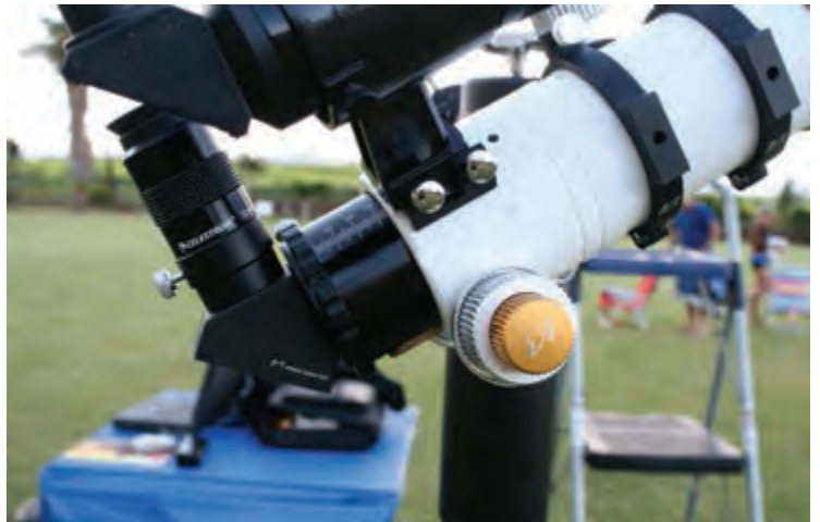
Image 3 - The William Optics Star 71 has a graduated drawtube with 35 mm of travel and includes a finderscope mounting base which can be positioned on either side of the tube.
