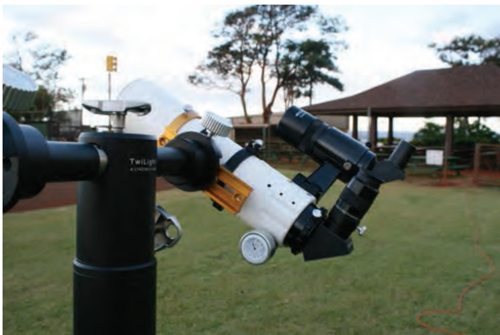
Image 1 - The beautifully crafted William Optics Star 71 five-element apochromatic refractor. Note the temperature gauge built into the focus knob.
