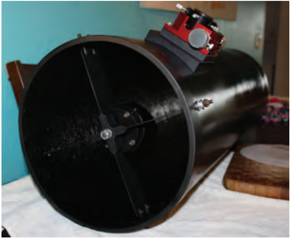
Image 9 - The author installed the MoonLite Model CR with the 1/2-inch plate to achieve proper spacing.
