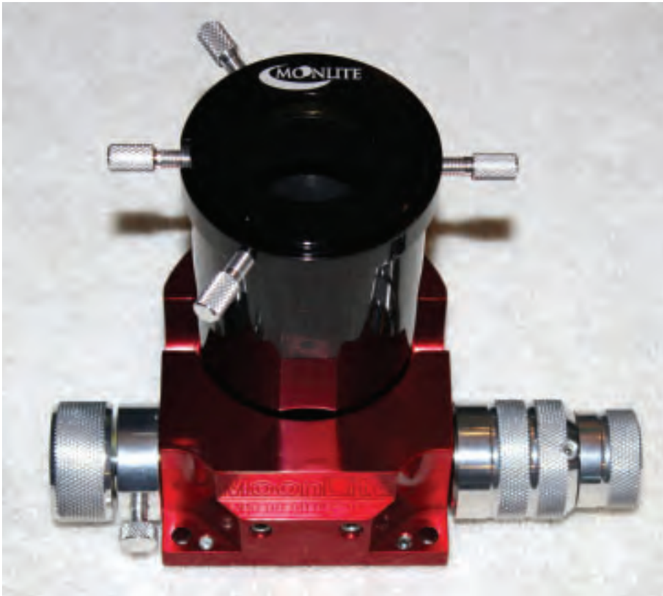
Image 1 - MoonLite Model CR Newtonian focuser with a 2.37-inch drawtube, three locking screws on the drawtube compression ring, a locking knob, and a 2 inch-to-1.25 inch adapter.
