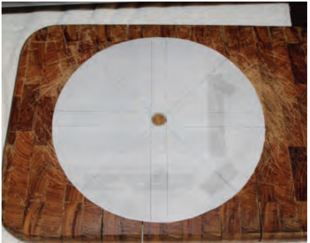
Image 10 - The primary mirror did not come from the factory with a center mark, so a template was made the same diameter as the mirror for positioning a DIY mark.
