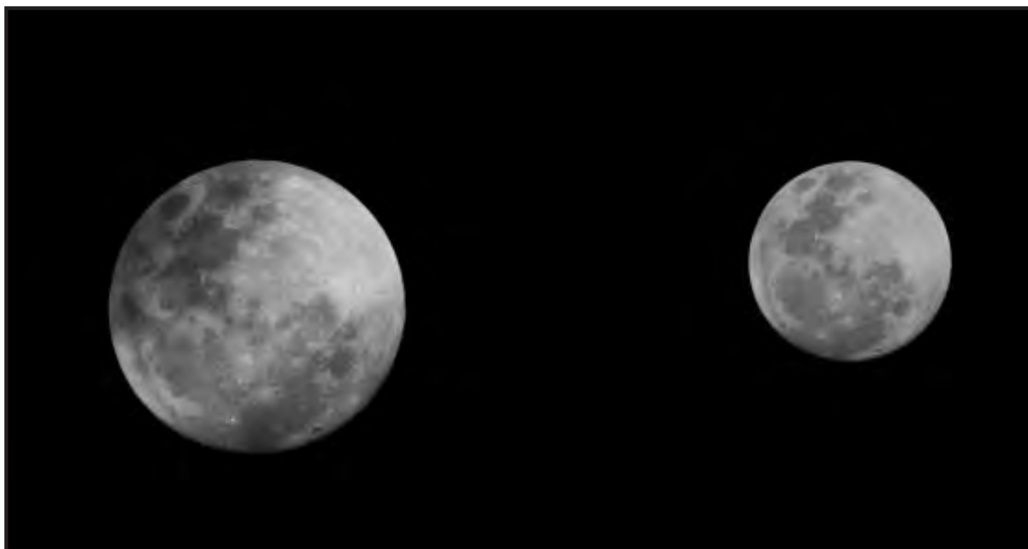
Image 3 - The nearly-full Moon imaged through both the GTF81 (right) and the GRF102 (left) with the same CCD camera, demonstrating the 47-percent increase in magnification achieved by the 102's 704-mm focal length.
