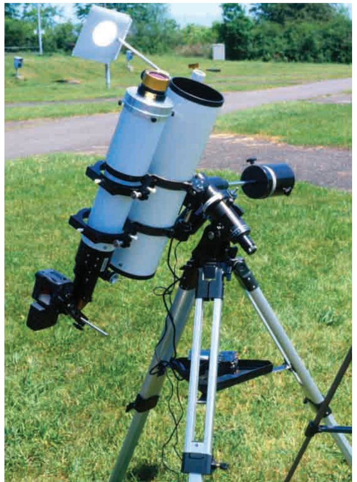
Image 1 - The author's 4.5-inch Newtonian projects the Sun onto a screen while he captured H-alpha images using the refractor on the same mount.
