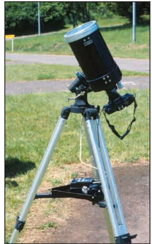
Image 3 - TPolar aligned and tracking the Sun, the author's SLR camera is attached to a 5-inch Schmidt Cassegrain telescope.
