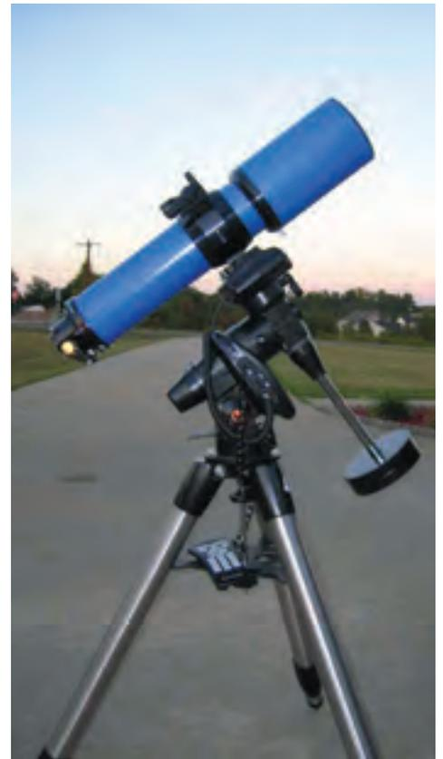
**Image 1 - The author's 4-inch apochromatic refractor mounted on an EQ-6 GEM.**
