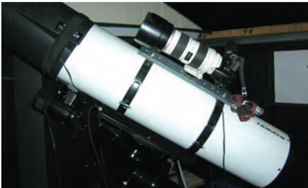
Image 2 - The Canon EF 70-200mm f/2.8L IS USM Lens mounted atop the telescope in the author's observatory, [www.wildwoodpines.org](http://www.wildwoodpines.org).
