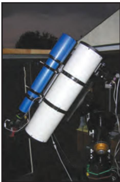
The Orion 190-mm Maksutov-Newtonian Astrograph in the author's observatory on a Parallax HD150 German equatorial mount with a 4-inch apochromatic refractor guide scope.
