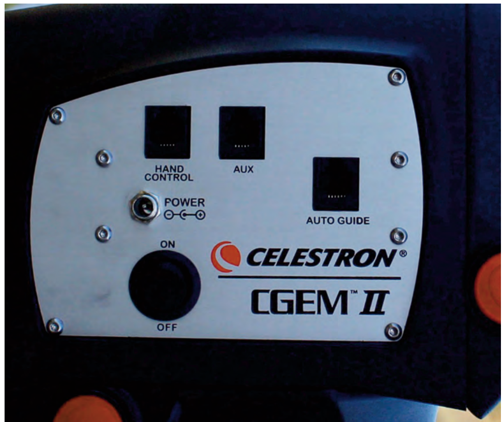
Image 4 - The side plate of the CGEM II mount head. The new white face makes it easier to see the labels at night.
