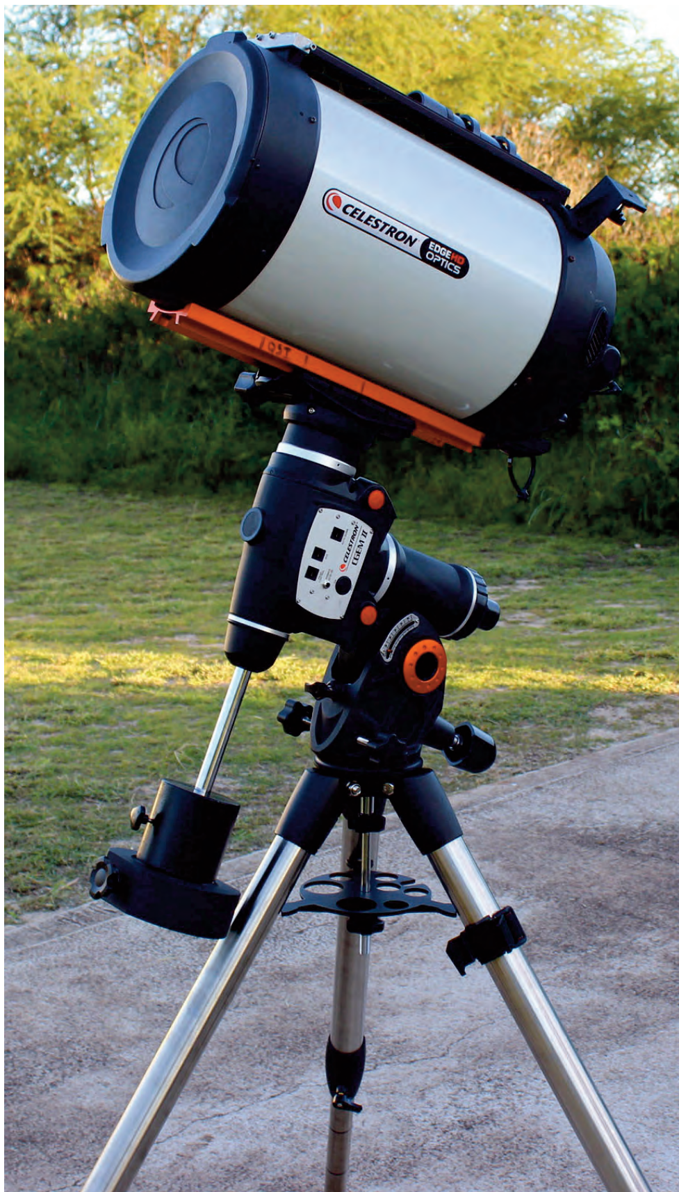
Image 7 - The mount is rated to hold a C11 telescope, as shown.
