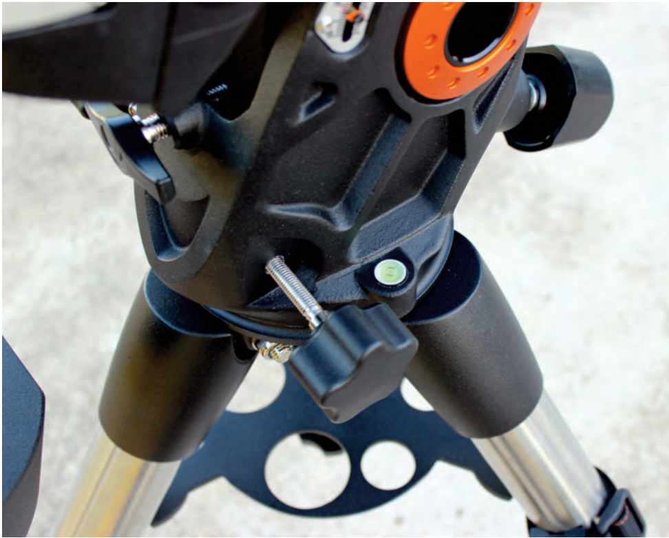
Image 5 - A bubble level is built into the mount and the azimuth adjustment knobs have large hand grips.
