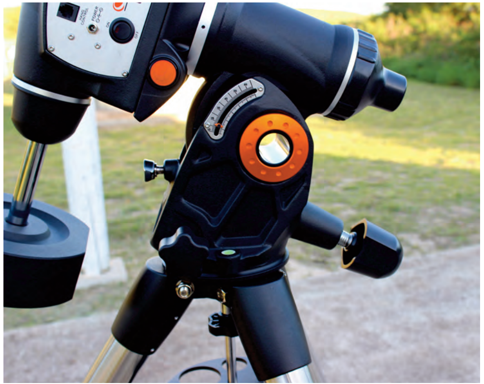
Image 6 - The latitude scale ranges from 15° to 70°. A large hand knob on the right makes it easy to raise the altitude of the mount, even with the maximum 40-pound payload aboard.
