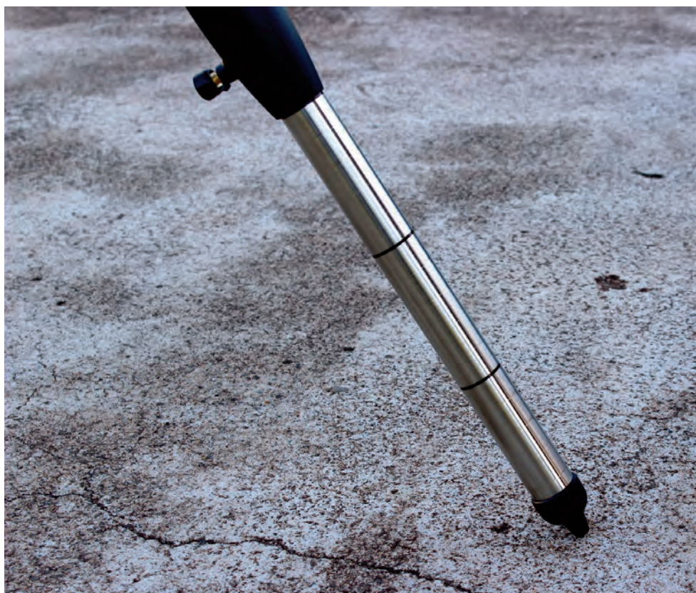
Image 2 - Close-up of the graduations on the tripod leg extensions. The marks are 5.0 inches apart.
