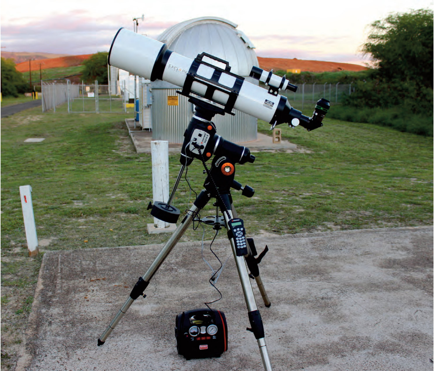
Image 8 - The author tested the mount with a 6.0-inch refractor powered with a 12-volt battery pack. The hand controller, the power cord, and the optional Celestron GPS unit are plugged into the side of the mount.
