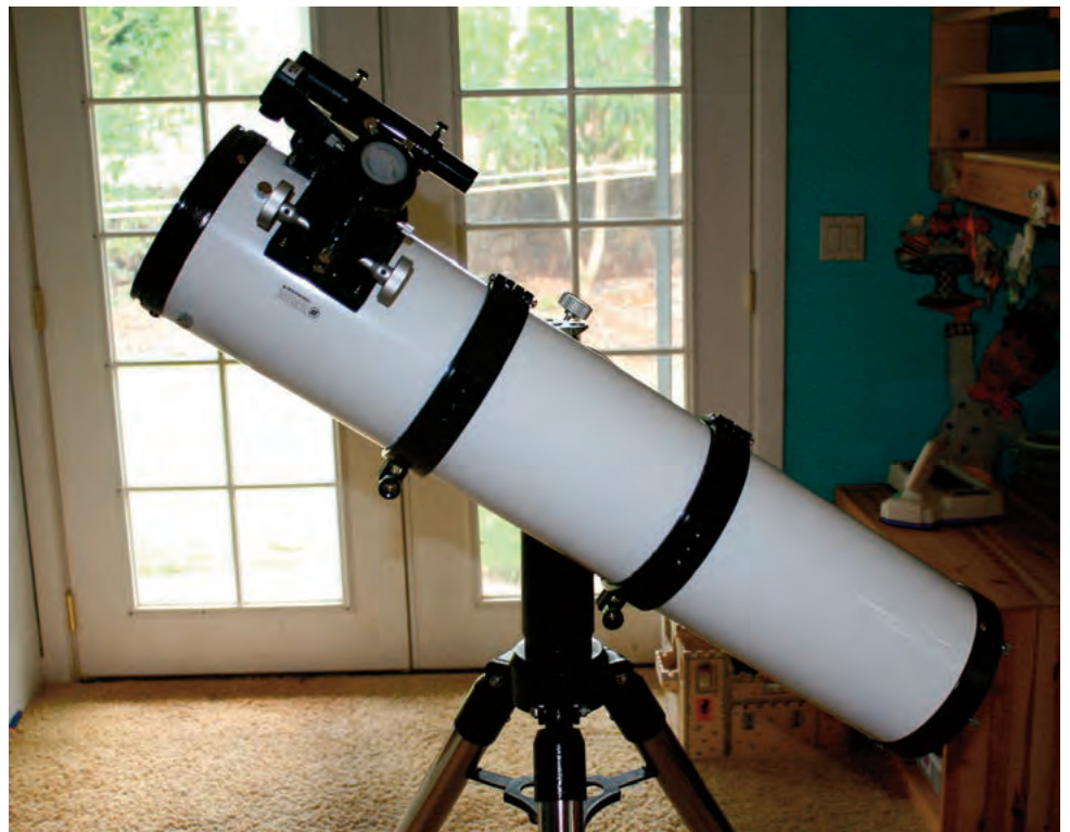
Image 1 - TPO 6-inch f/6 Newtonian on an Explore Scientific Twilight II alt-azimuth mount
