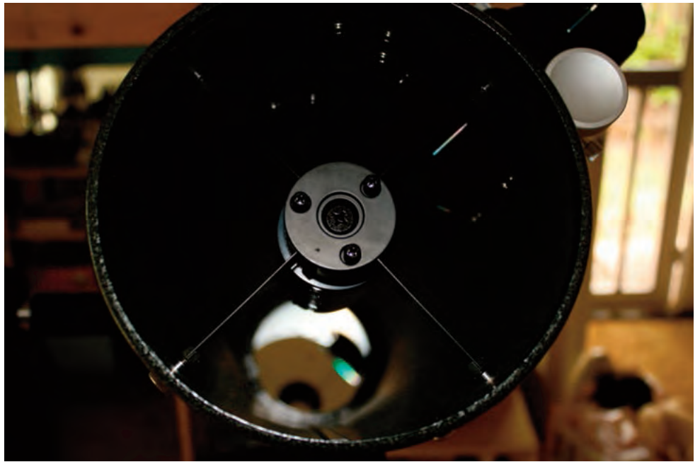
Image 3 - The secondary mirror assembly is a four-vane style that is adjusted via three Phillips-head screws.
