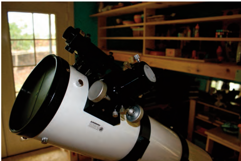
Image 2 - The reviewed version of the 6-inch f/6 TPO Newt is equipped with a single-speed 2-inch focuser. OPT reports that the current version carries a dual-speed 2-inch Crayford-style focuser.
